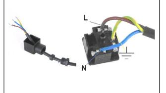
**9.** Place the connector gasket on the connector, and plug the connector on the timer as shown below, and tighten the screw (maximum 1Nm). Make sure that the two gaskets are
